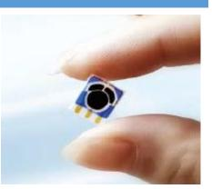
The sensor is composed of three catalytic electrodes, a solid electrolyte, and gas diffusion holes. The gas reaches the working electrode of the sensor through the diffusion holes, an electrochemical redox reaction occurs on the porous micro-surface of the electrode, the solid electrolyte conducts electron transfer, and generate a current signal as an output. The current signal can characterize the gas concentration.
